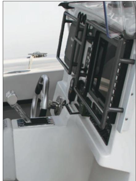
*Hand supports around these touch-screens facilitate the drags and taps necessary for precise operation of the electronics even in rough sea conditions.*
