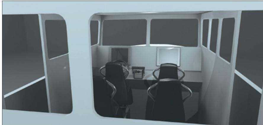
*The cabin dashboard in an enclosed helm station should have the same dimensions and orientation as those discussed for the console. Cabin structure will further limit visibility from an enclosed helm, and adequate space for operators and passengers to move around the seats must be a design consideration.*
