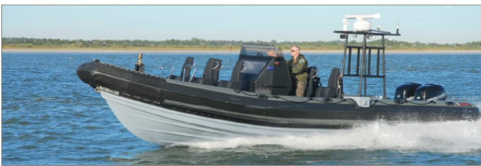
**Left**—A well-designed composite console will push air to the sides and over the top with a minimum of resistance and resulting turbulence. A low windscreens installed at a slight negative angle can eliminate wind in the helmsman’s face by pushing air high enough to flow over the head. **Right**—This Brunswick 1000 Impact model RIB sports a well-designed aluminum console with flat faces angled to push aside wind and spray when operating at speed.
