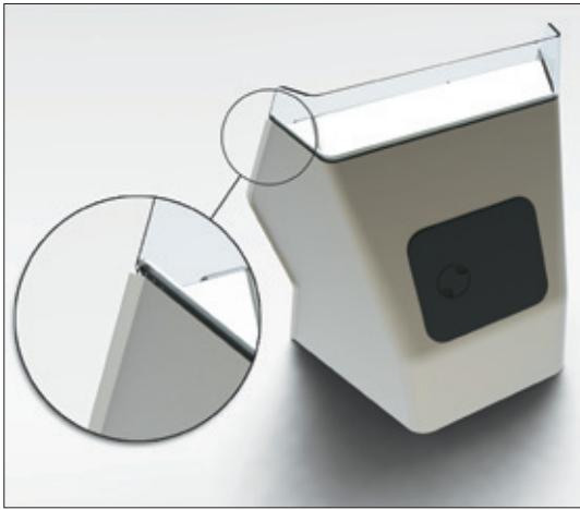
**Left**—Placing helmsman and navigator side by side puts two sets of eyes on the water, a real advantage during high-speed operations in rough weather or sea conditions. It also facilitates nonverbal communication and enables two people to reach the boat controls in the event of an accident or injury. **Right**—A slight “kick” angle at the trailing edge of the console will help deflect wind and spray.
