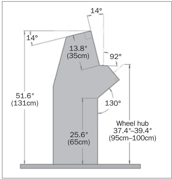
*Shown in profile, this generic helm console provides good visibility forward, convenient location of navigation screens, easy access to the helm and throttle control, and ample space for feet and legs, even in rough conditions.*
