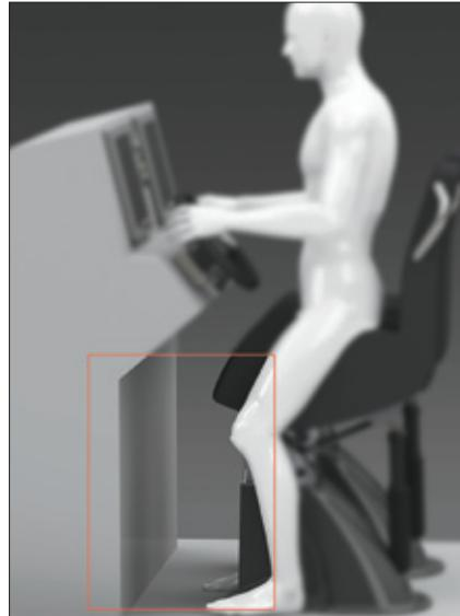
**Left**—Below the helm and throttle plane, the console should be cut away (about 45° from vertical) to provide space for the operator's knees to flex. The area should be clear of obstructions such as ignition or power switches, which the knees might hit during operation. **Right**—The vertical rear surface down to the deck should be at least 11.8" (30cm) forward of a vertical line through the center of the helm.
