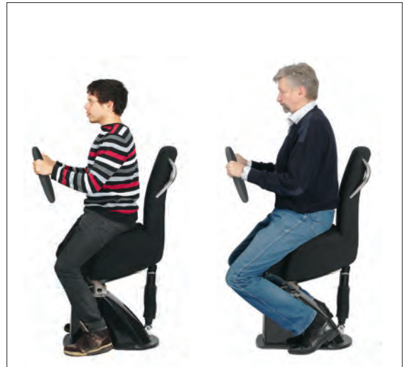
Left —Because height of the eyes is largely a function of leg length, vertical adjustment is not necessary, even on the helmsman's seat. Here, the eyes of a 5'1" (157cm) person land just below the shoulder of the 6'6" (199cm) author when the two are standing. The eyes of those same individuals seated on a straddle seat are at nearly the same height. Similarly, slight variations in the bend of arms and legs make longitudinal adjustment of straddle seats unnecessary in a well-designed helm station. Right —A seated 5'6" (167cm) person is compared to the author.
