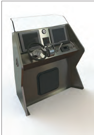
Left —Placing helmsman and navigator side by side puts two sets of eyes on the water, a real advantage during high-speed operations in rough weather or sea conditions. It also facilitates nonverbal communication and enables two people to reach the boat controls in the event of an accident or injury. Right —A slight “kick” angle at the trailing edge of the console will help deflect wind and spray.
