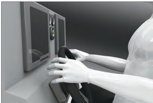
Left —The wheel should be mounted so the steering column points toward the operator's shoulders. That way, any bracing force applied by the helmsman during high-speed operations will be in the same general direction as the wheel shaft. Right —Orient throttle controls so that at cruising speed they point straight up; this allows for better fine adjustment by a hand at about elbow level.
