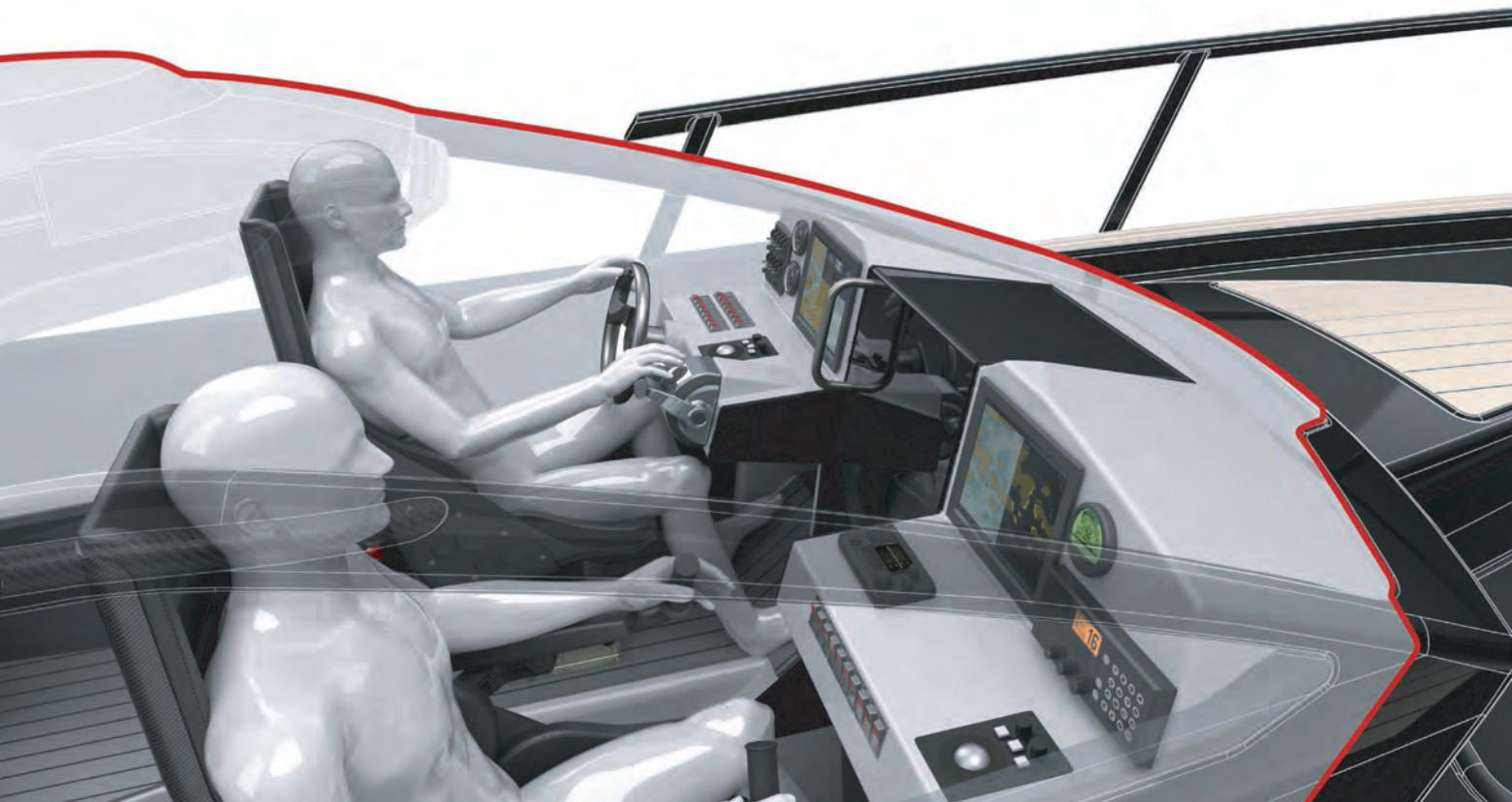
Bucket seats require longitudinal seat adjustment for the driver, legroom under the dash, and careful consideration of the limited sight lines from a low sitting posture.
