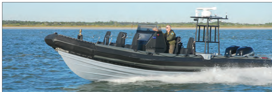
Left —A well-designed composite console will push air to the sides and over the top with a minimum of resistance and resulting turbulence. A low windscreen installed at a slight negative angle can eliminate wind in the helmsman’s face by pushing air high enough to flow over the head. Right —This Brunswick 1000 Impact model RIB sports a well-designed aluminum console with flat faces angled to push aside wind and spray when operating at speed.
