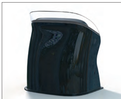
Left —A well-designed composite console will push air to the sides and over the top with a minimum of resistance and resulting turbulence. A low windscreen installed at a slight negative angle can eliminate wind in the helmsman’s face by pushing air high enough to flow over the head. Right —This Brunswick 1000 Impact model RIB sports a well-designed aluminum console with flat faces angled to push aside wind and spray when operating at speed.
