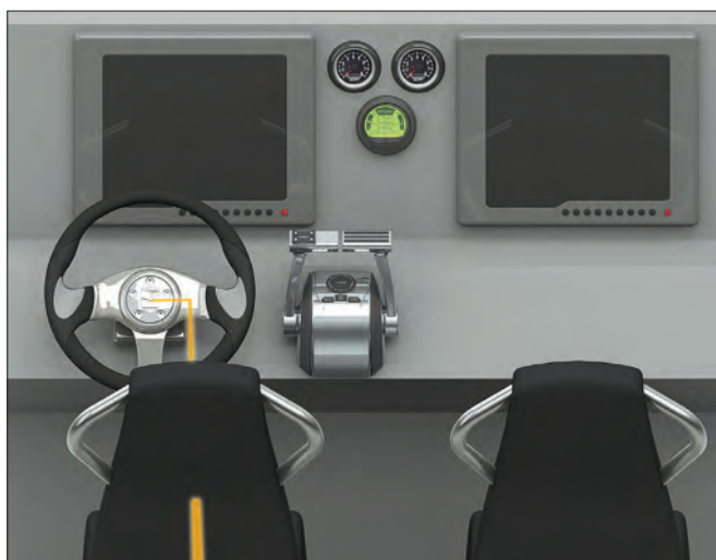
Left —Below the helm and throttle plane, the console should be cut away (about 45° from vertical) to provide space for the operator's knees to flex. The area should be clear of obstructions such as ignition or power switches, which the knees might hit during operation. Right —The vertical rear surface down to the deck should be at least 11.8" (30cm) forward of a vertical line through the center of the helm.
