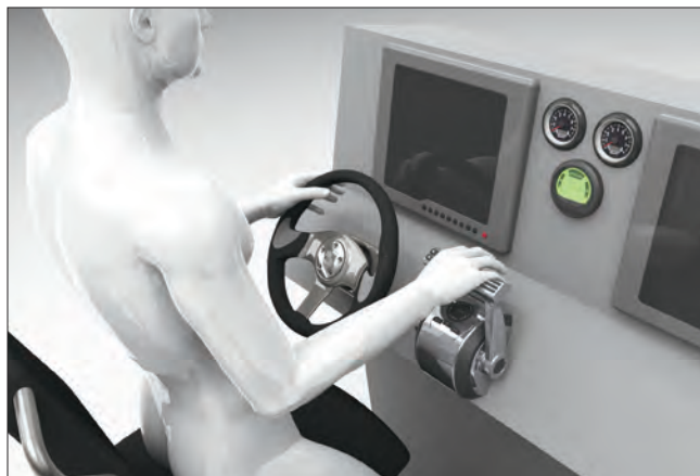
Left —The wheel should be mounted so the steering column points toward the operator's shoulders. That way, any bracing force applied by the helmsman during high-speed operations will be in the same general direction as the wheel shaft. Right —Orient throttle controls so that at cruising speed they point straight up; this allows for better fine adjustment by a hand at about elbow level.
