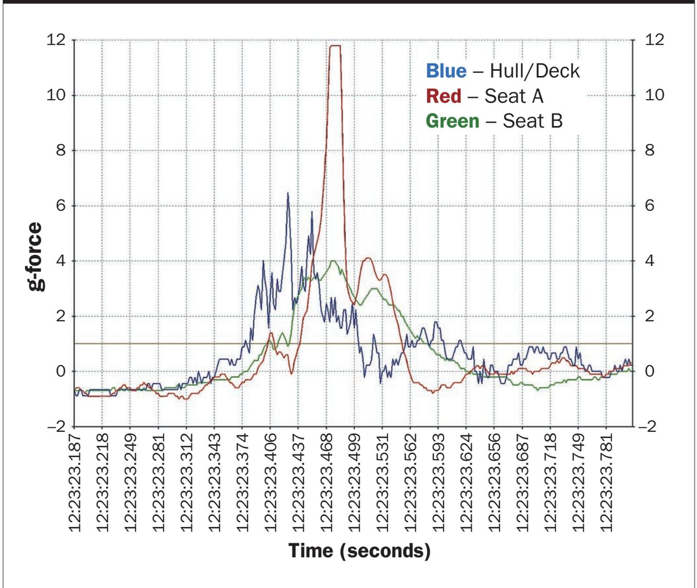
Overlay of the highest recorded impact suggests that the crew member in Seat A was subjected to more than 12 g. Note that the limit for the accelerometer was 11.5 g, thus the flat peak of the graph. Extrapolation of the graph indicates a peak in excess of 14 g.
