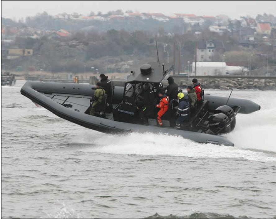
Designers at Boomeranger tested two models of shock-mitigating seats to determine which better dampened the vertical and lateral accelerations crews are likely to be exposed to in high-speed, rough-water operations. The seats were installed in the forward position ahead of the helm station, and the crew riding in them were monitored as the boat was run through a variety of maneuvers in different wind and sea states.
