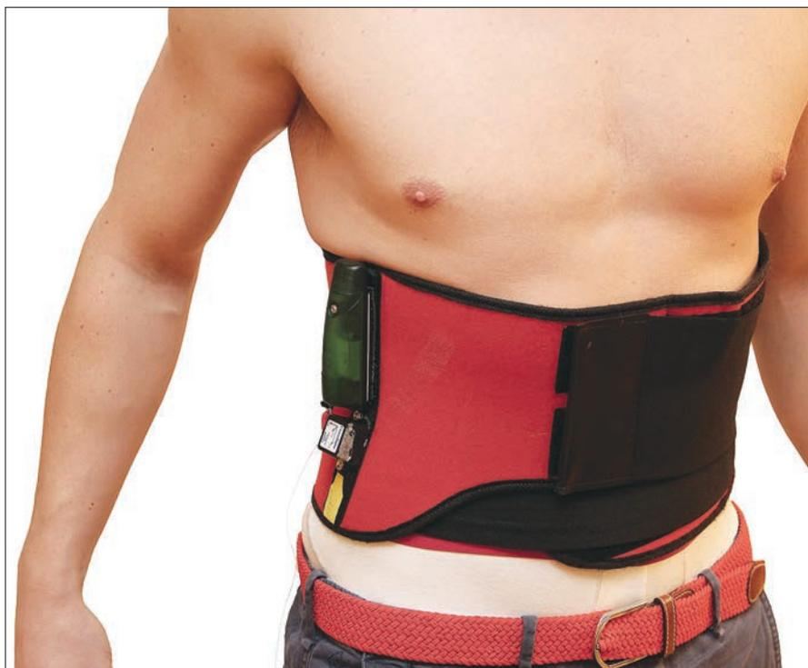
*To measure the forces on the crew, the accelerometers were bound tightly to their torsos in kidney belts worn inside survival suits. The method has been validated against bone-anchored sensors and was found to be suitably accurate for impacts up to 16–20 Hz.*
