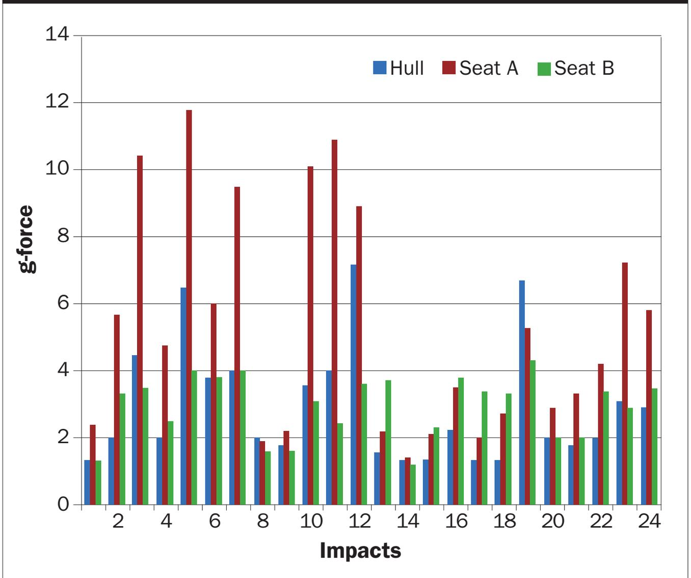
Accelerometer readings of the 24 highest impacts were isolated from the broader data to focus on how two shock-mitigating seats handled them. Data reveal instances in which Seat A seemed to amplify the impacts delivered to the hull.
