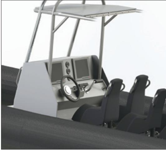
*Locate the supporting legs of a T-top far enough apart that they do not overlap and create a visual obstruction wider than 2.2" (55mm).*
