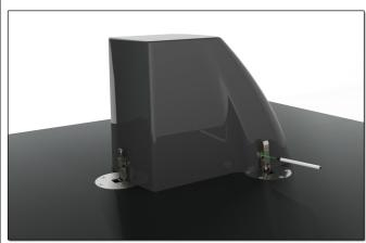
2: Place the jockey pedestal over the plates. The pedestal overlaps the plates equally.
