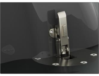
4: Mount the eccentric locks with 3x M4 bolts / lock. Mount in combination with large washers inside the pedestal.
