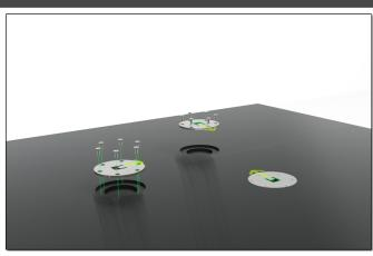
1: Place the fixture plates in position on deck. Each plate fastens with 6x M6 counter sunk. Place the plates with the "U" shape facing inwards (towards the pedestal)
