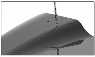
3: Drill the marked holes. The lower holes may require counter sinking the internal flange for placement of washers and nuts.
