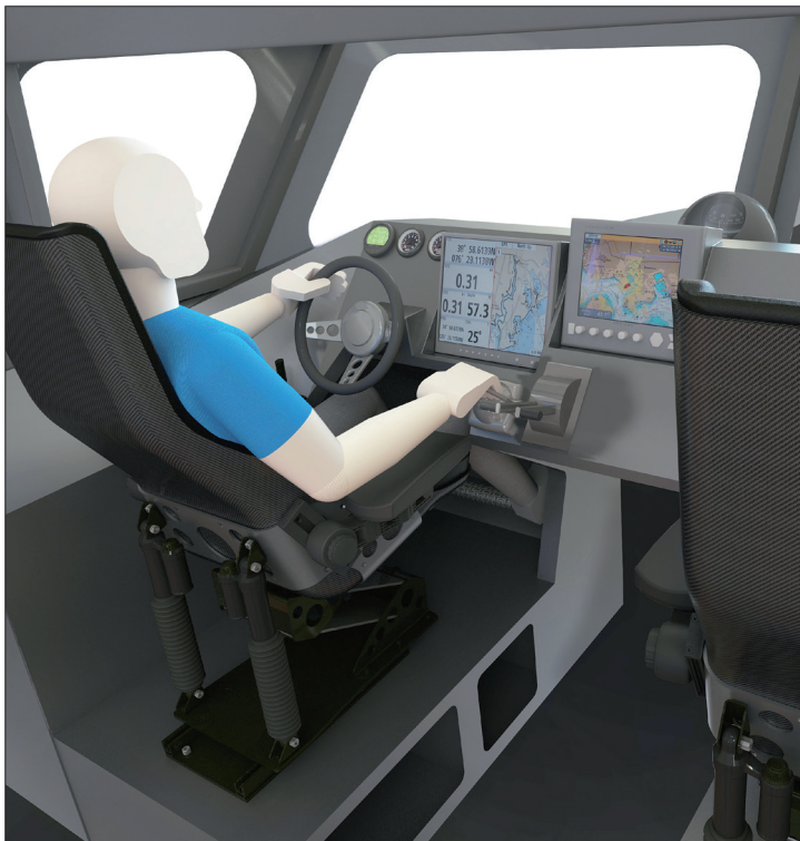
Bucket seats require longitudinal seat adjustment for the driver, legroom under the dash, and careful consideration of the limited sight lines from a low sitting posture.
