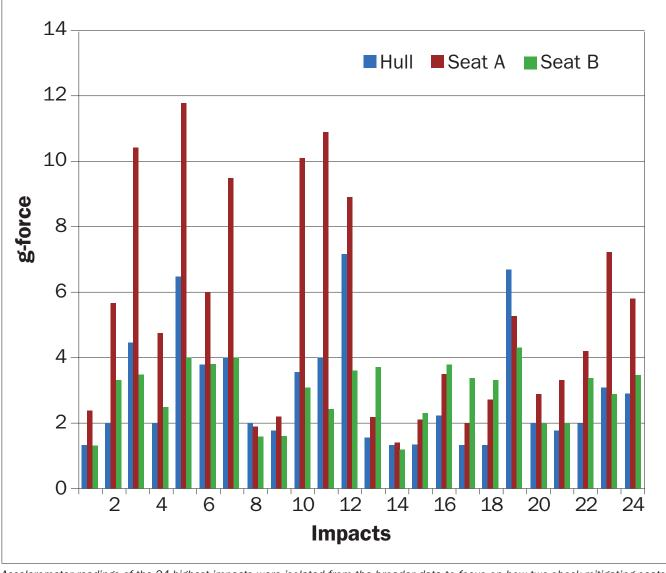
Accelerometer readings of the 24 highest impacts were isolated from the broader data to focus on how two shock-mitigating seats handled them. Data reveal instances in which Seat A seemed to amplify the impacts delivered to the hull.
