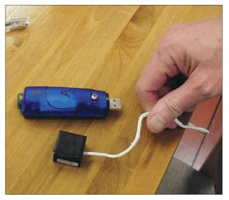
Data were collected through multiple accelerometers and data loggers attached directly to the deck inside the console to measure hull impacts, and strapped to the crew to measure impacts transmitted up through the seats.
