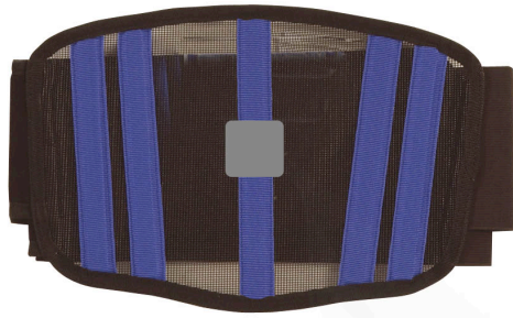
Fig. 2. Girdle keeping accelerometer fixed on back.
