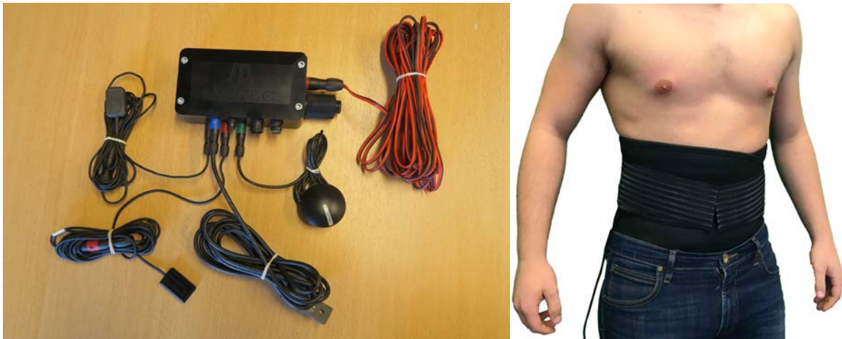
Figure 6 The Marec data logger, connected with (counter-clockwise) two human accelerometers, the hull accelerometer, the GPS antenna, and the red/black power cord. Kidney belt with the accelerometer attached as close as possible to crista iliaca (upper edge of the pelvis) on the axillar line (side line).
