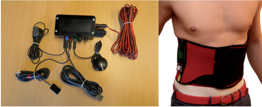
Figure 6. The Marec data logger, connected with (counter-clockwise) two human accelerometers, the hull accelerometer, the GPS antenna and the red/black power cord. A kidney belt is attached with the sensor as close as possible to crista iliaca (top of the upper edge of the pelvis) on the axillar line (side line).
