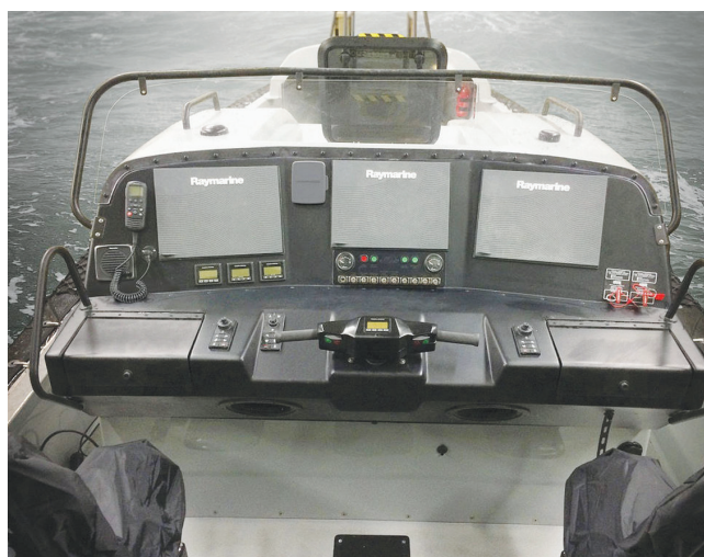
The Ullman Steering Bar System, installed on Norsafe's Magnum 850 craft Harald Bluetooth ; the system enables coxswains to steer, throttle and simply hold on to the bars, simultaneously
